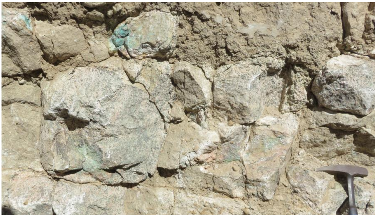
Set of steeply-dipping 'sheeted' A-veins exposed in N-S trench near DDH-010 collar.
